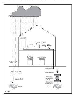
Washing machines and dishwashers should be connected to the FOUL drainage system, the water will then be taken to a sewage works for treatment before being discharged safely into a river.
